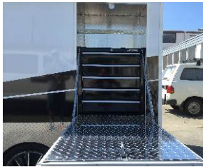
SET BACK DIVIDER: PUSHES BIKES BACK TO CREATE WALK IN ACCESS TO THE TRAILER WITH RELOCATABLE WHEEL SUPPORTS. (UNIQUE TO MOTOSTAR)
