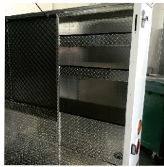
SET BACK DIVIDER: PUSHES BIKES BACK TO CREATE WALK IN ACCESS TO THE TRAILER WITH RELOCATABLE WHEEL SUPPORTS. (UNIQUE TO MOTOSTAR)
