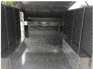
INTERNAL ALUMINIUM MESH LINING POWDER COAT BLACK OR MILL FINISH
