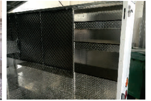
REMOVABLE SET BACK DIVIDER, PUSHES BIKES BACK TO CREATE WALK THRU ACCESS INTO TRAILER. WHEEL STOPS CAN BE POSITIONED ON SHELF OR DIVIDER
